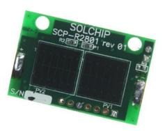
Saelig Company, Inc. has introduced the patented Sol Chip Pak<sup>™</sup> (SCP-R2801). Their Power Modules offer day/night non-stop functionality by combining state-of-the-art solar cells, a rechargeable battery, and advanced power management circuitry. These power modules include all the components that are required to harvest energy from ambient light, charge a built-in rechargeable battery, and deliver a stable voltage to a load. <u>Read more...</u>
